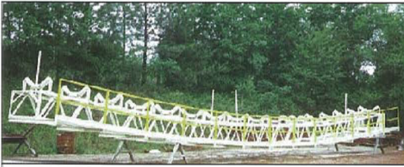
CURVED CONVEYOR SECTION FOR RADIAL STACKER
