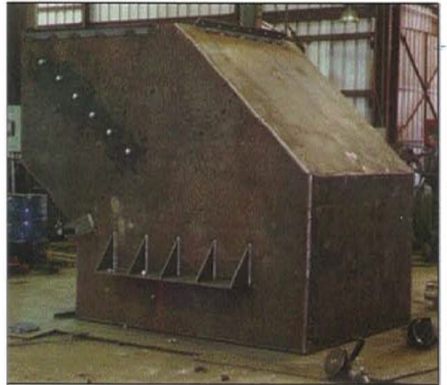
CONVEYOR HEAD CHUTE
