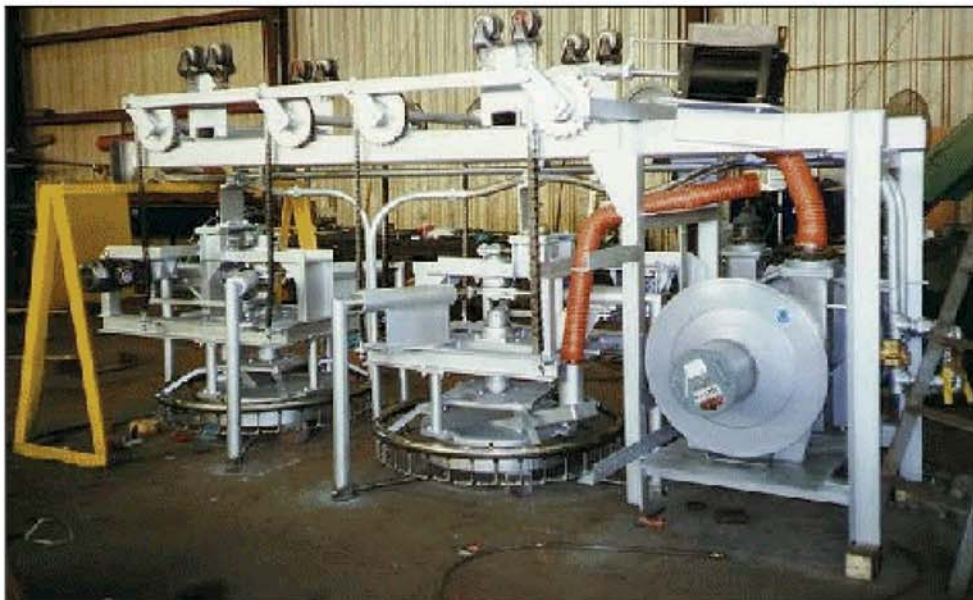
RAIL WHEEL TREAD QUENCH MACHINE BUILT PER CUSTOMER DESIGN
