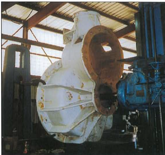
73" RAYMOND® ROLLER MILL GEAR HOUSING BEING REPAIRED
