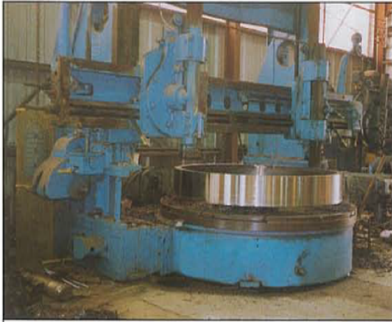
MACHINING SLEEVE FOR 73" RAYMOND® ROLLER MILL BASE
