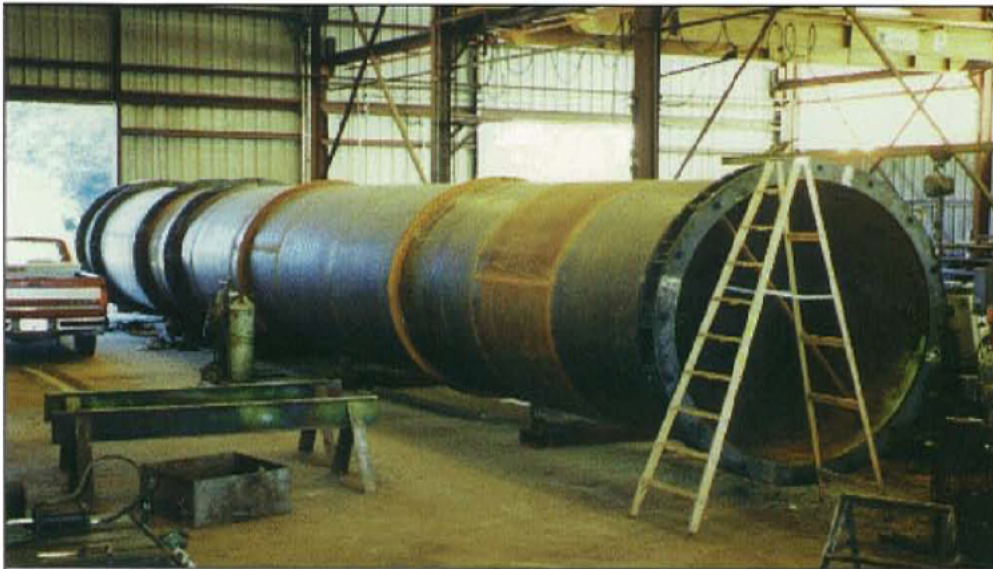
8' X 60' CONVEYOR SUPPORT COLUMN
