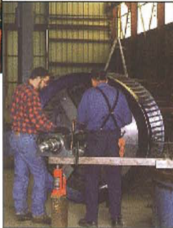
CLASSIFIER HOUSINGS BEING SET UP TO MACHINE & ASSEMBLY OF CLASSIFIER ROTOR
