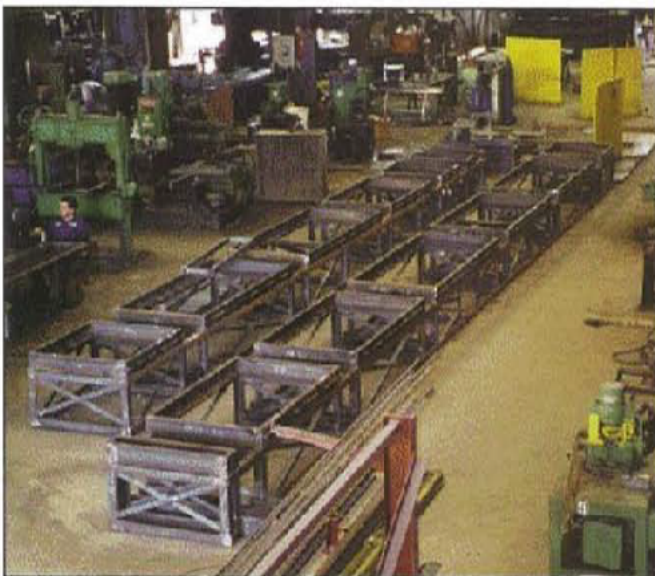
FITTING & WELDING CONVEYOR FRAMES
