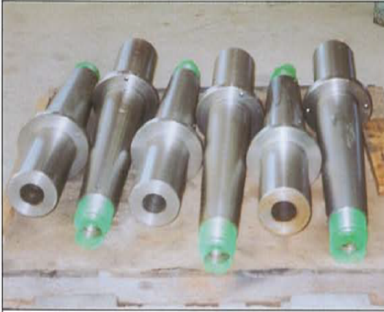
66" JOURNAL SHAFTS MACHINED & READY TO SHIP OUT TO CUSTOMER
