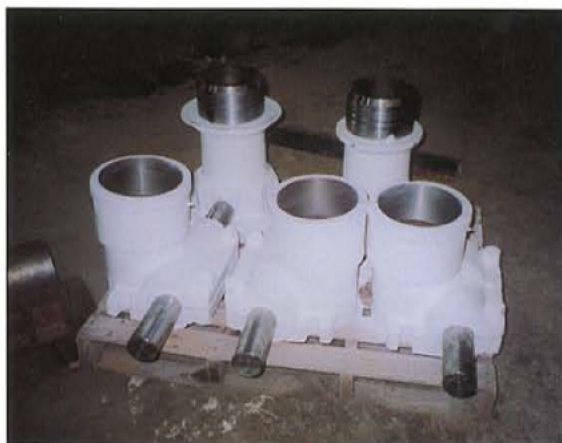
REPAIRED JOURNAL HEADS FOR 73" MILL
