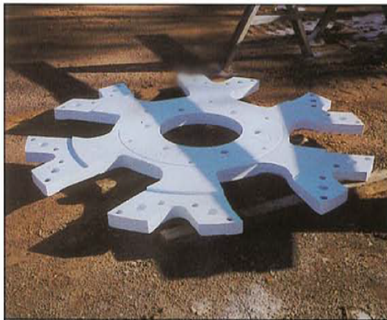
FABRICATED SPIDER PLATE FOR 73" RAYMOND® ROLLER MILL
