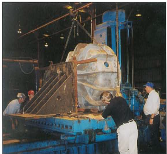
73" RAYMOND® ROLLER MILL GEAR HOUSING BEING REPAIRED
