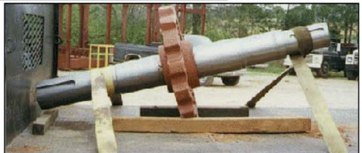
HEADSHAFT DRIVE ASSEMBLY FOR BUCKET ELEVATOR
