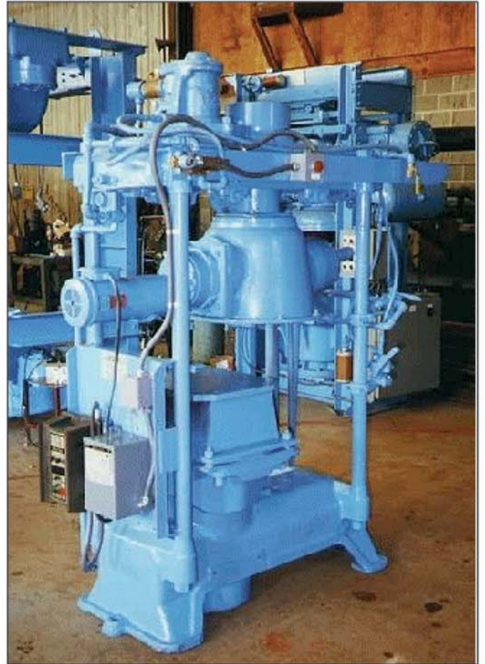
FOUNDRY CORE BLOW MACHINE AFTER BEING REBUILT & UPGRADED
