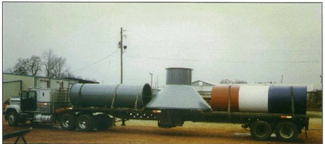
SCRUBBER STACK & CONE BASE
