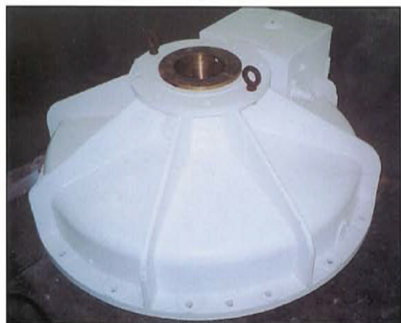
REPAIRED 50" MILL GEAR HOUSING
