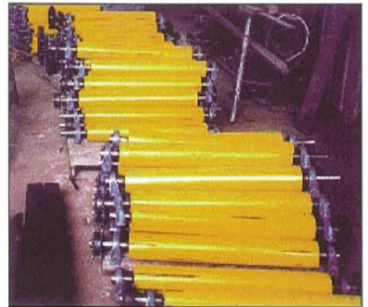
CONVEYOR ROLLS ASSEMBLED WITH BEARINGS
