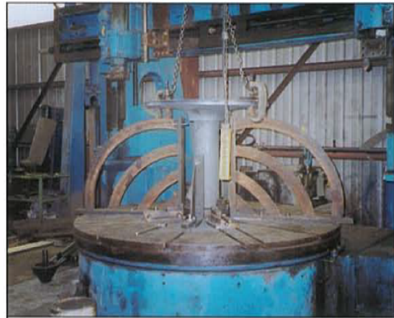
50" MILL BOTTOM CASTING BEING MACHINED
