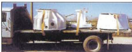
REPAIRED 73" MILL GEAR HOUSING REPAIRED 66" PLOW SUPPORT NEW FABRICATED WHIZZER SECTION
